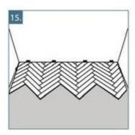
15. For the following rows, begin by installing the A-Panels from left to right, then complete the row by placing the B-Panels from right to left.
