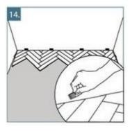
14. Place spacers between the flooring and the wall to maintain a 10mm expansion gap.
